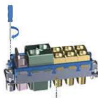
装配好模块后, 闭合滑动边框, 锁上螺丝 After finished assembly, close sliding border, lock screw
